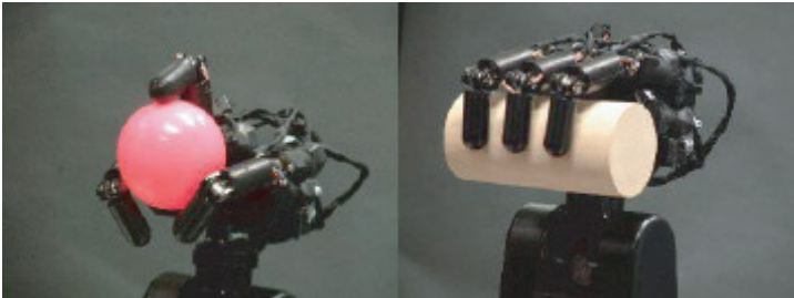
Fig. 1.4 The enveloping grasp of the high-speed multi-fingered robotic hand
