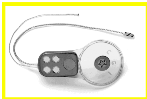
Figure 6.6. The ABI implantable system consists of a receiving antenna, a hermetically sealed electronics package that receives and decodes the signal, and a current source stimulator, and the electrode array.
