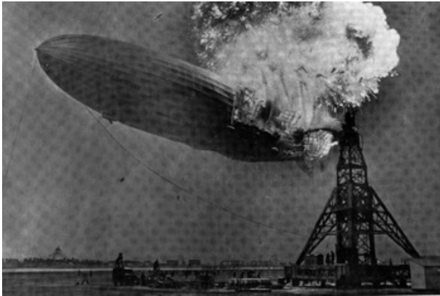
Fig. 8. In New Jersey in 1938, during the process of mooring the Hindenburg zeppelin to the mast, the Hindenburg exploded and burned. The Hindenburg used hydrogen for lift. There are many explanations of the cause of the explosion.
