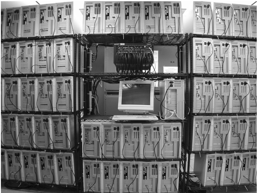
Figure 1-4: 128-Processor Beowulf cluster built by Donald Becker while he was at NASA/GSFC (reprinted with permission Michigan Technological University).
