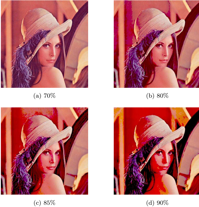
Fig. 2. Example of compression Lena image by means hard thresholding putting to zero 70% (a), 80% (b), 85% (c) and 90% (d) of wavelet coefficients
