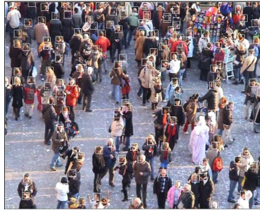
Fig. 9. Left figure: snapshot of the software interface developed to detect the individual dynamics from a video recording during the Venetian Carnival 2007.
