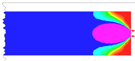
Fig. 1.5. St. Venant's principle: local effects quickly die out.
