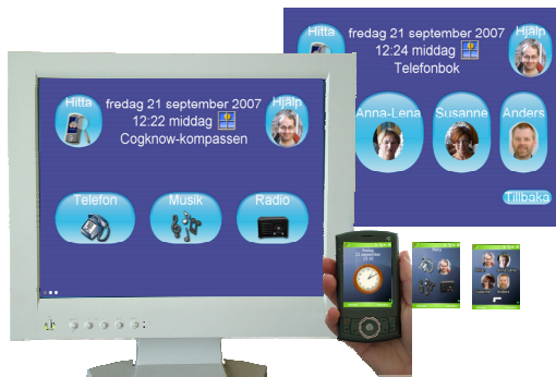
Figure 5 [15] (right). A smart schedule reminder developed in COGKNOW project.
