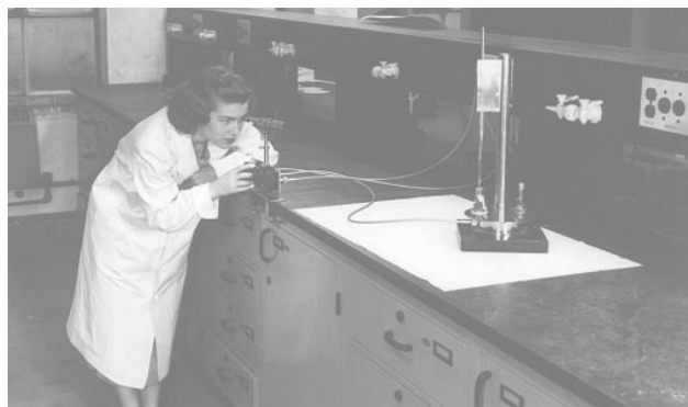
Fig. 5. Darleane Christian, Spring 1950 photo at Ames Laboratory, with remote apparatus for pipetting radioactive solutions.
