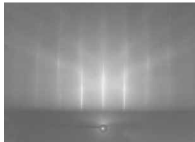
Fig. 5. RHEED image for as grown GaN surface measured after air exposure.
